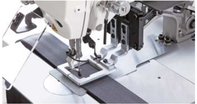
Example application: Reinforcing the stitching of seatbelts *The feeding frame is a special order item.
