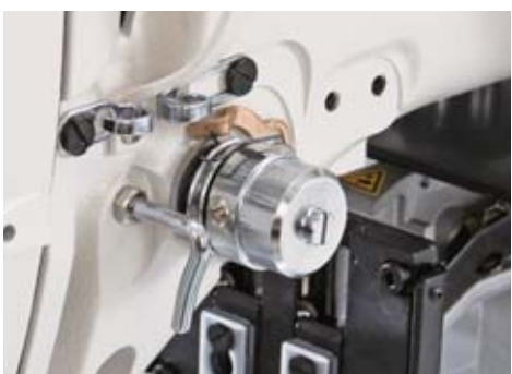
The intermediate presser goes up and comes down according to the material thickness.
