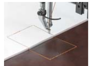
The height of the intermediate presser is constant.
