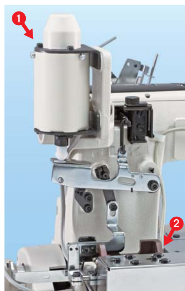
① Presser lifter drive mechanism ② Thread trimmer drive mechanism
